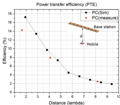
Fig. 3. PTE graph of the simulation and measurement
