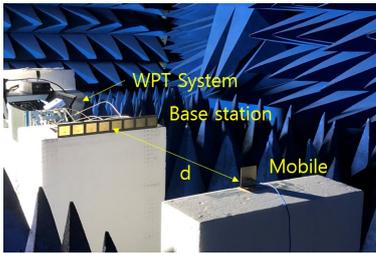
Fig. 2. The MPT measurement setup
